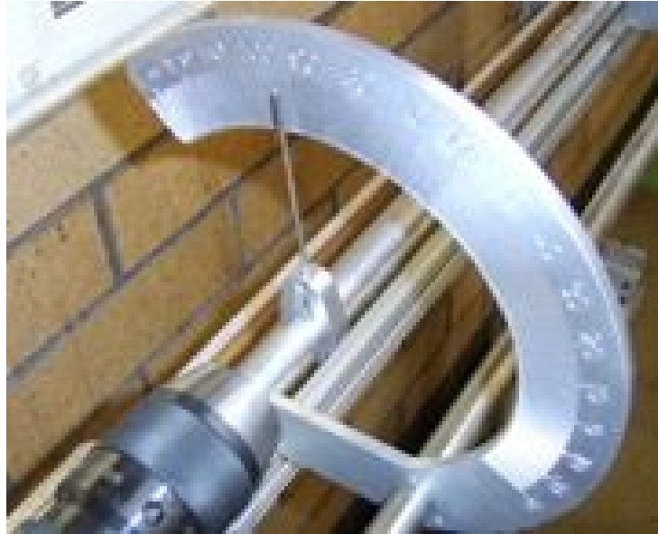
Figure 2. Chuck vise, pointer, and protractor scale.
